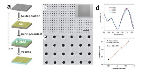
Figure (a) Schematic for transfer of Au nanohole arrays from the Si template to PDMS substrates. (b,c) SEM and optical images of the nanohole array transferred to PDMS. (d) Transmission spectra and sensitivity of the fabricated nanohole array sensor.
