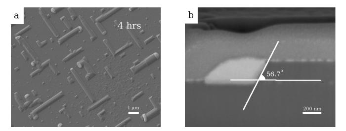
**Figure 1.** a) SEM planar views of Si wires obtained on Si(100) substrate at T = 650 °C using 1nm Au film annealed at 600 °C for 30 min. The Si deposition time is indicated on the figure. b) High resolution SEM image of the Si wire cross-section performed with focused ion beam along the growth direction. The theoretical value for the liquid-solid interface oriented along Si (111) direction is 54.7°
