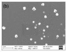
Figure 1 (a) and (b): Chitosan nanoparticle images captured through SEM at the Western Nanofabrication Facility
