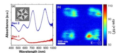
**Figure 1. (a)** Absorption measurements of a fivebranched dendrimer for generations 1 and 2 (generation 2 in the inset, scale bar is 200 nm). The SHG activity for a five-branched generation 2 is shown in **(b)**.
