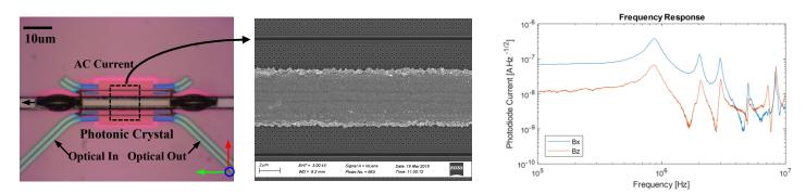
*Fig. 1* (a) Optical image of device after BHF etching showing the optical I/O, deposited metal, and photonic crystal region (b) LEO 1530 SEM image of region indicated with 5  $\mu$ m wide patterned Silver/Chromium microwire (c) Dynamic response of the photonic crystal membrane under two different external magnetic field orientations.
