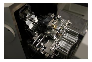
The new 5-Axis stage. The stage accepts sample holders for mounting stubs, wafer pieces and full 4-inch wafers.
