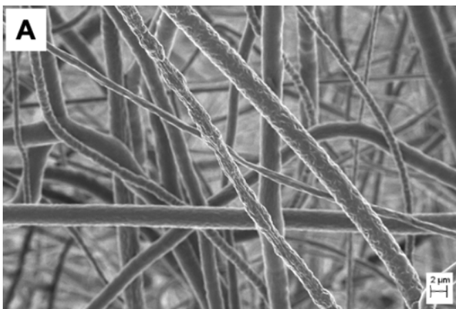
Figure 1. hPDL infiltrated the full thickness of the semi-permeable scaffold. (A,B) Electrospun polycaprolactone (PCL) nanofibers with sodium tripolyphosphate (STPP) and chitosan coating.
