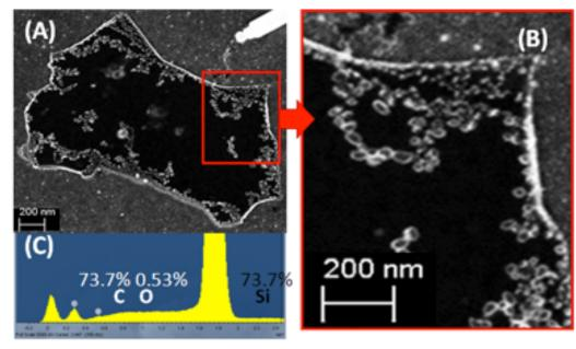
(A) SEM Inlens image of nano-pores (white and hollow dots) on graphene film on silicon substrate and (B) its magnified image. (C) EDX spectrum on the pores
