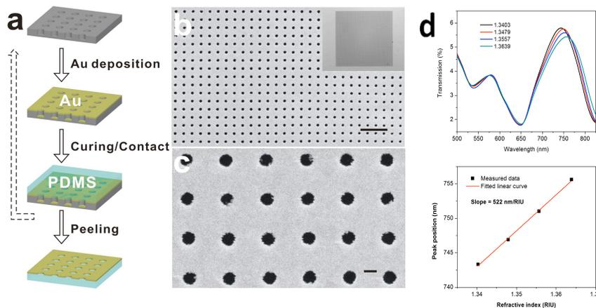
Figure (a) Schematic for transfer of Au nanohole arrays from the Si template to PDMS substrates. (b,c) SEM and optical images of the nanohole array transferred to PDMS. (d) Transmission spectra and sensitivity of the fabricated nanohole array sensor.
