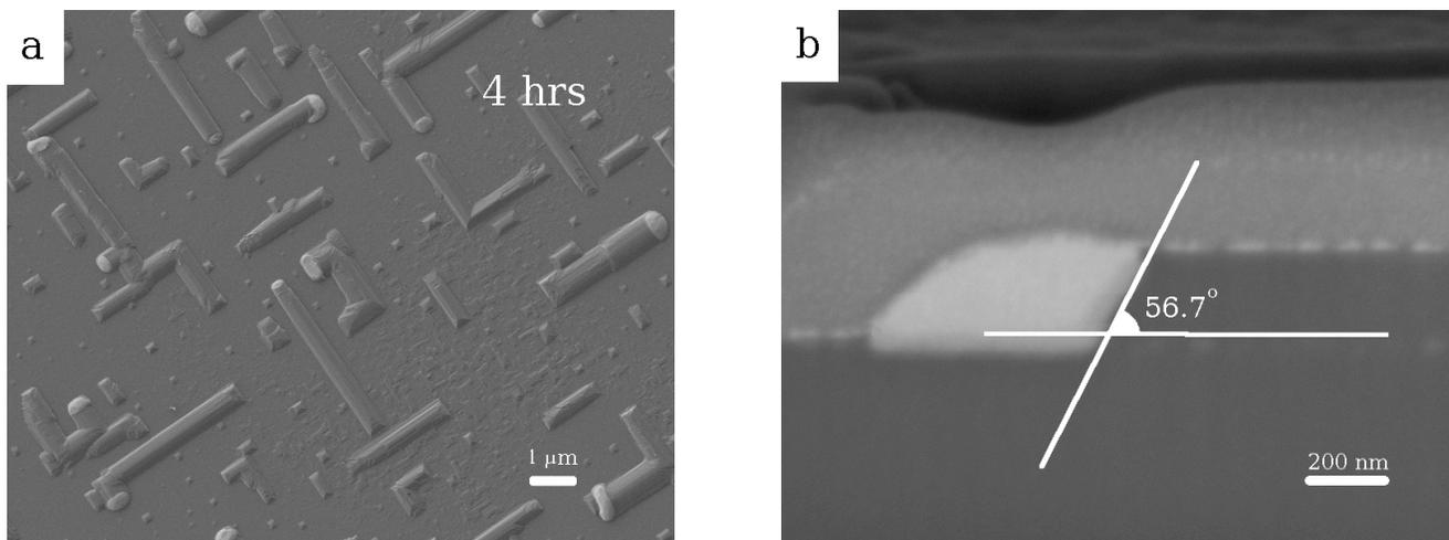
**Figure 1.** a) SEM planar views of Si wires obtained on Si(100) substrate at  $T = 650\text{ }^{\circ}\text{C}$  using 1nm Au film annealed at  $600\text{ }^{\circ}\text{C}$  for 30 min. The Si deposition time is indicated on the figure. b) High resolution SEM image of the Si wire cross-section performed with focused ion beam along the growth direction. The theoretical value for the liquid-solid interface oriented along Si (111) direction is  $54.7^{\circ}$
