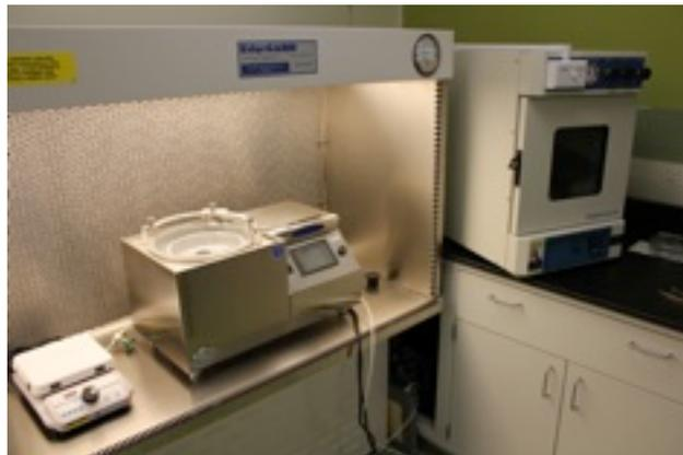
Laminar Flow Bench with Spinner and Vacuum Oven
