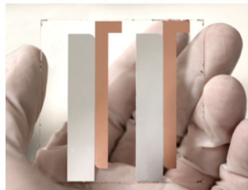
Figure (a) The 2D cross-section of a DBD plasma actuator. (b) Bottom view of a MEMS plasma actuator shows the aluminium coating of the grounded electrode while the copper layer of the exposed electrode can be seen through the glass substrate.
