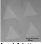
Figure 2: Optical image of triangular windows in the polymer surface
