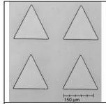
Figure 1: Optical image of the photoresist triangles
