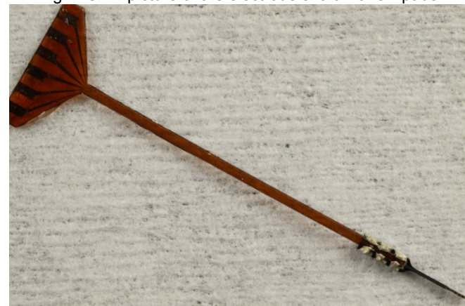
Fig-4. Single-shaft electrode and flexible cable assembly
