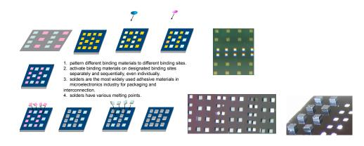
The substrate with various binding sites was patterned with Karl Suss MA6 Mask Aligner; SU8 covers was also patterned Karl Suss MA6 Mask Aligner; Solder coverage and assembly process were carried out in heated DI water with a hotplate;
