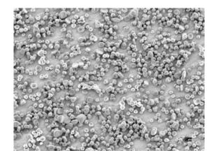
**Figure 3.** Coaxially electrosprayed core-shell microspheres for controlled drug delivery. Scale bar =  $20\mu m$ .
