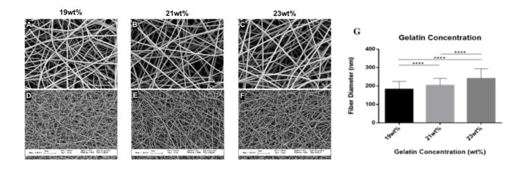
*Figure 2.* Effect of varied solution concentration on fiber diameter. A-F) Representative images of scaffolds 7500x magnification (A-C, scale bar =  $1\mu$ m) and 1500x magnification (D-F, scale bar= $10\mu$ m). G) Average fiber diameter in response to varied gelatin concentrations. N=3, n=450, one-way ANOVA, p<0.05. Data represented as mean ± SD.
