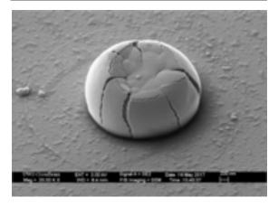
*Figure. 2.* SEM images of the deformed 2200 nm spheres under 0. 01 loading rate
