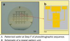
The grafted polymer layers were patterned and depositioned with sub-micron fidelity using a combination of photolithography and UV-GP (above). A thin layer of aluminum is deposited in Step B of the photolithographic sequence, acting as an adhesive layer for the photoresist.
