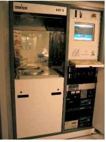
Deep Reactive Ion Etching (DRIE) of silicon is one of the key processes required for MEMS, microsystems, and sensor development. Applications typically require high aspect ratios, etch depths of as great as  $500 \mu$ m, etching through-the-wafer, etching into a buried cavity in the wafer, or etching onto buried oxide.
