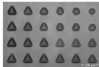
**Figure 2.** Bright field optical image of water droplets localized in the triangular glass areas.
