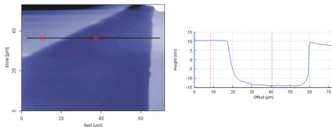
**Figure 4.** AFM image (a) and cross-section image (b) taken across a triangle window in the fluoropolymer background.
