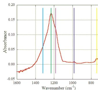
**Figure 3.** FTIR spectrum of the fluoropolymer film deposited on a silicon wafer.
