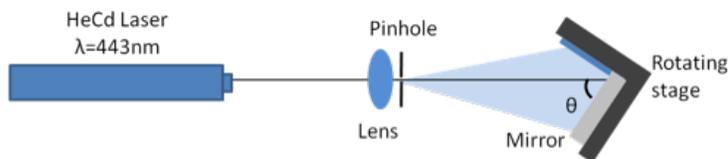
Figure 1 - Illustration of Lloyd's mirror interferometer setup
