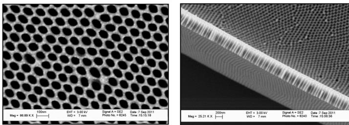
**Figure 3.** SEM images of PAA implanted with Au ions. (A) Cross-sectional, elevated view of implanted film with a uniform bright layer, indicating Au ion penetration into the mask. (B) Plan view of PAA displaying the segregated Au ions as bright clusters.
