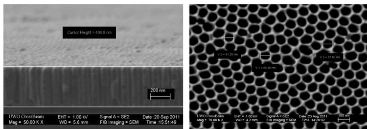
Figure 2. SEM images of porous anodic alumina synthesized at 40 V in 0.3 M oxalic acid for four minutes. (A) Cross sectional view of PAA displaying pore height; wall thickness appears exaggerated due to osmium coatings. (B) Plan view of PAA indicating the pore diameter of 85±5 nm.
