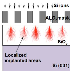
Figure 1. Schematic of ion implantation with the nanoporous alumina mask
