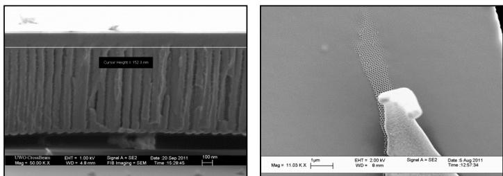
**Figure 4.** SEM images of PAA implanted with Si ions. (A) Cross sectional view of PAA showing the depth of morphological changes to the surface structure. (B) Plan view of implantation through debris, contrasting the implanted and non-implanted sites.
