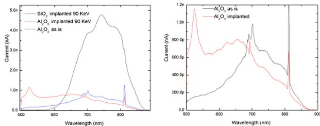
**Figure 5.** Photoluminescence spectra of unimplanted and implanted  $\text{Al}_2\text{O}_3$  compared to  $\text{SiO}_2$  matrix. (from permission of R. D'Ortenzio)
