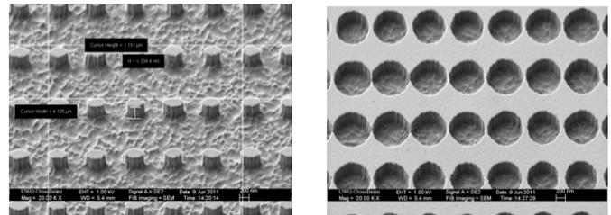
Figure 2 - SEM image of a nano-pillar array (left) and a nano-hole array (right)
