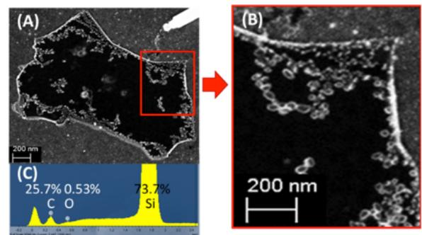
**Figure (A)** *Sem in lens image of nano-pores (white and hollow dots) on graphene film on silicon substrate and (B) its magnified image. (C) EDX spectrum on the pores.*
