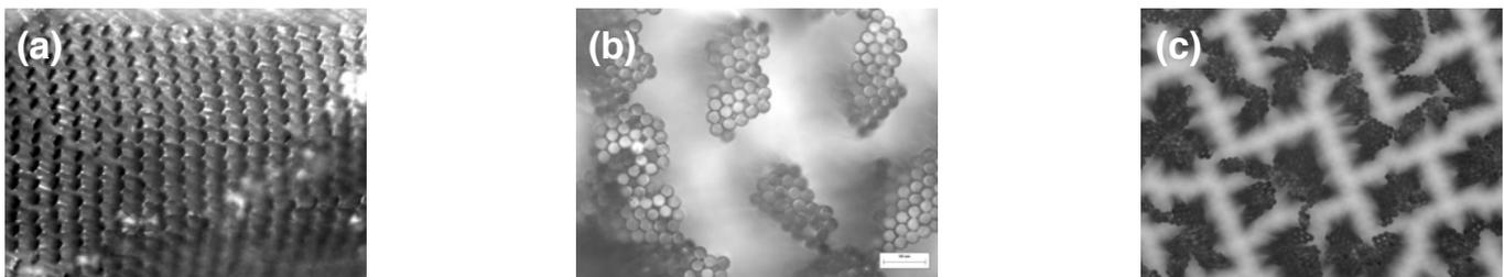
**Figure 1** Optical microscopic images of (a) SU-8 pillars collapse after blow-drying by air gun. (b)-(c) SU-8 pillars bend and stick to each other after drying by natural evaporation
