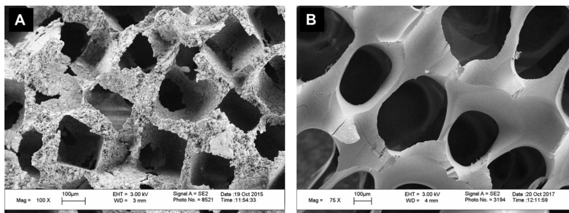
**Figure 1.** SEM images of porous bone tissue engineering scaffolds. A) Scaffolds made of polycaprolactone/ (borophosphosilicate glass) hybrid through solvent-free casting and particulate leaching; B) 3D printed scaffolds of polyvinylpyrrolidone/(calcium phosphosilicate glass) hybrid materials.
