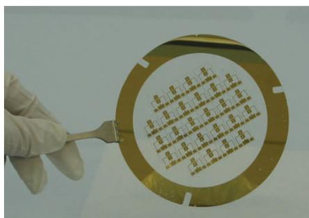
the capacitor pads on the substrate and the teeter-totter structure of the common plate must be very closely aligned and have a gap of 4-13µm between them.
