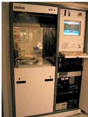
Deep Reactive Ion Etching (DRIE) of silicon is one of the key processes required for MEMS, microsystems, and sensor development. Applications typically require high aspect ratios, etch depths of as great as 500  $\mu\text{m}$ , etching through-the-wafer, etching into a buried cavity in the wafer, or etching onto buried oxide.
