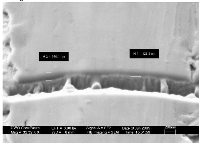
to provide cross sectional cuts to be further studied with SEM. An example of a tilt corrected FIB milling cross section observed with the SEM, is shown in Figure 3. The thickness was shown to average about 180 nm with a variation of  $\sim 60$  nm (averaged over 10 pads that were milled) [2].
