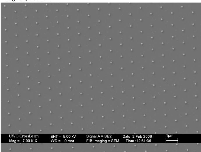
to 100 nm (see *Figure 2*). The Au-templated samples are then used for the growth of NW arrays, using McMaster's molecular beam epitaxy facilities.
