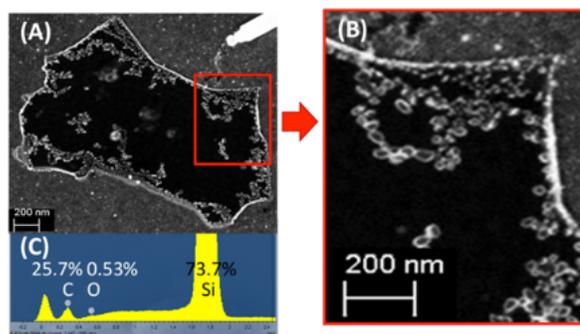
**Figure (A)** *Sem in lens image of nano-pores (white and hollow dots) on graphene film on silicon substrate and (B) its magnified image. (C) EDX spectrum on the pores.*
