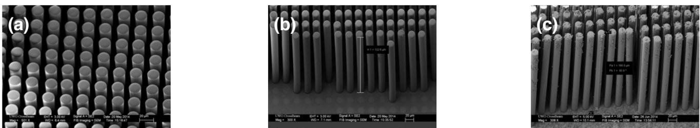
**Figure 2** (a) SEM results of high aspect ratio SU-8 pillars fabricated by the critical-point-dry assisted photolithographic process. (b) aspect ratio of 9:1 (c) aspect ratio of 11:1
