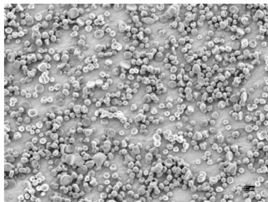
**Figure 3.** Coaxially electrospayed core-shell microspheres for controlled drug delivery. Scale bar = 20 $\mu$ m.
