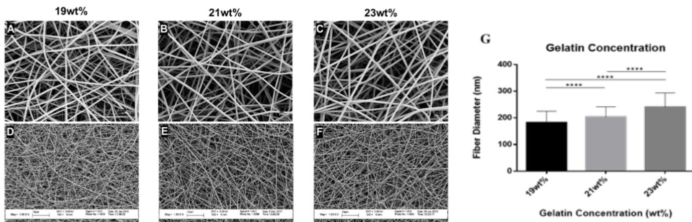
**Figure 2.** Effect of varied solution concentration on fiber diameter. A-F) Representative images of scaffolds 7500x magnification (A-C, scale bar = 1 $\mu$ m) and 1500x magnification (D-F, scale bar=10 $\mu$ m). G) Average fiber diameter in response to varied gelatin concentrations. N=3, n=450, one-way ANOVA,  $p < 0.05$ . Data represented as mean  $\pm$  SD.
