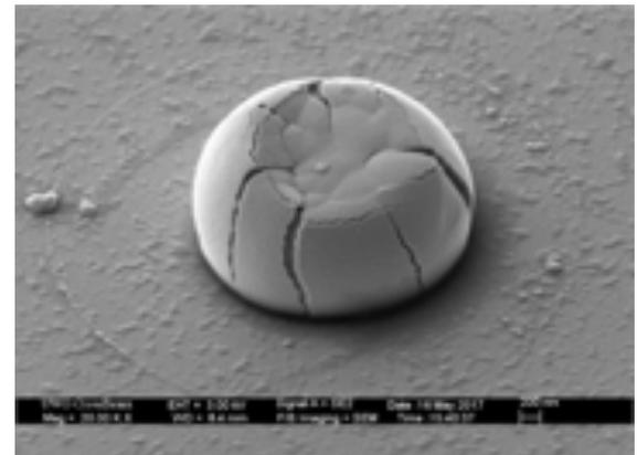
**Figure. 2.** SEM images of the deformed 2200 nm spheres under 0.01 loading rate
