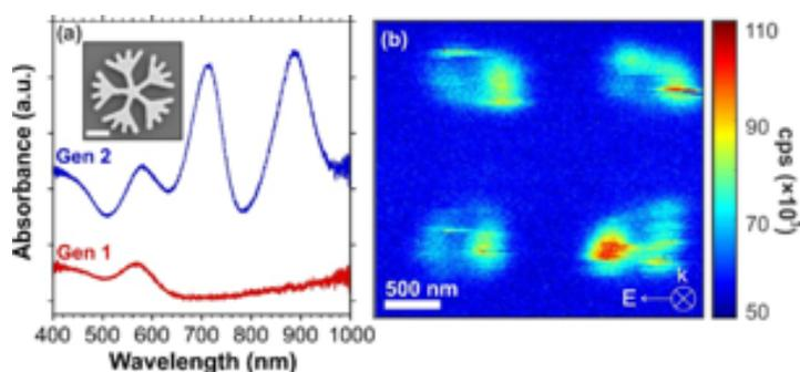
**Figure 1.** (a) Absorption measurements of a five-branched dendrimer for generations 1 and 2 (generation 2 in the inset, scale bar is 200 nm). The SHG activity for a five-branched generation 2 is shown in (b).
