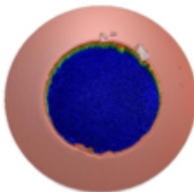
**Figure 2.** A 3d reconstruction of the electrode.
