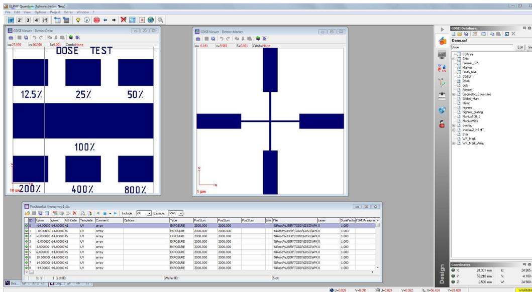
The e-beam lithography system has also been upgraded with the installation of the Raith Elphy Quantum system. The new software provides user friendly writing of patterns from CAD drawings in electron beam sensitive resist. The patterns can then be transferred to the substrate with subsequent etching or deposition processes.
