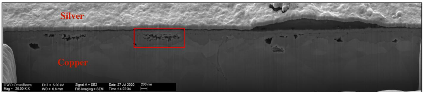
The FIB cut of a cold-spray copper coupon that was embedded in bentonite clay (compacted to a dry density of 1.1 g/cm<sup>3</sup>) for three months is shown above.
