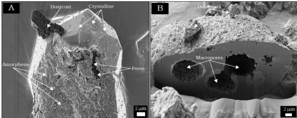
**Figure 1:** a) Typical features of a Glaciogenic particle collected in southern Iceland and b) Focus ion beam scanning electron microscopic (FIB-SEM) images of the internal structure of a 65µm Eyjafjallajökull Ash particle after FIB milling.
