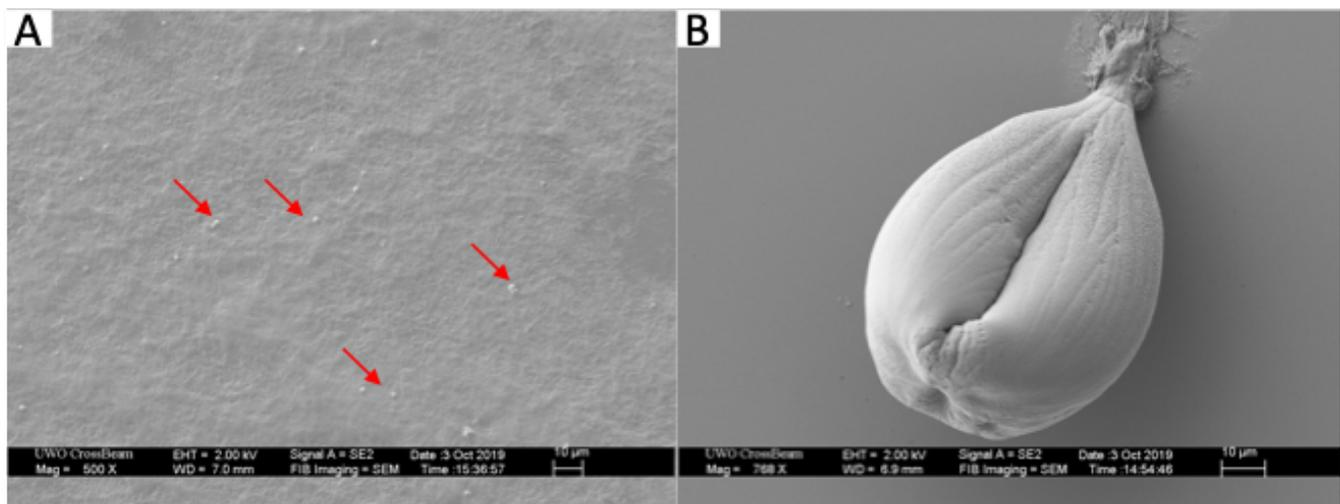
**Figure 1.** (A) SEM image of PVA-SiNP nanocomposite gel (red arrow pointing towards SiNPs). (B) SEM image of a PVA-SiNP-IONP microbead (before performing any freeze-thaw cycles).
