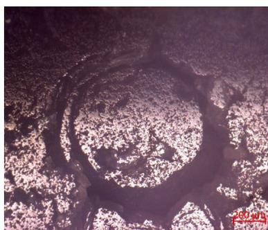
**Figure 2:** Microscope image showing an etched ring that appears on the surface
