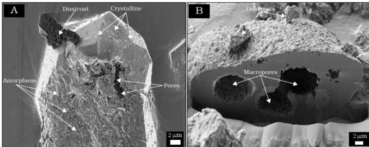
**Figure 1:** a) Typical features of a Glaciogenic particle collected in southern Iceland and b) Focus ion beam scanning electron microscopic (FIB-SEM) images of the internal structure of a  $65\mu\text{m}$  Eyjafjallajökull Ash particle after FIB milling.
