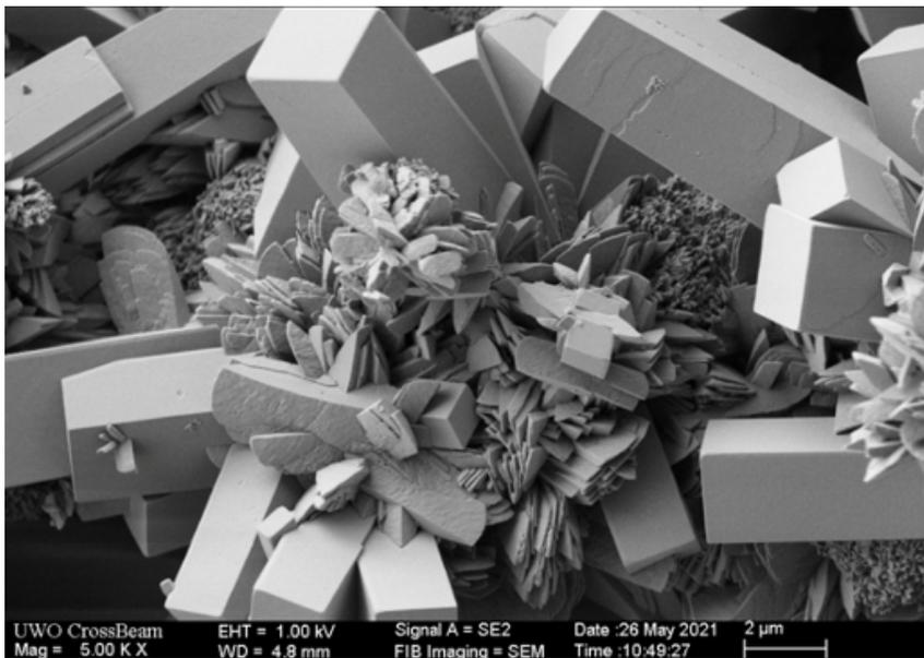
**Figure 2:** SEM Imaging of Calcium Phosphate (Organic Precursor) on Titanium Nanotubes via ECD
