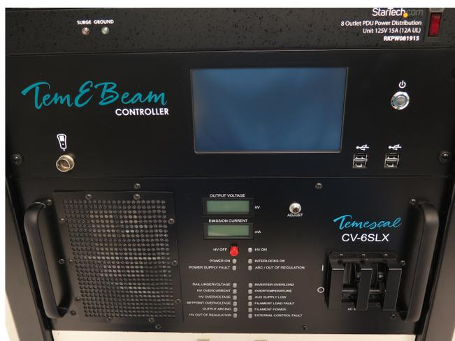
*Temescal CV-6SLX 10kV 6 kW Power Supply and Beam Controller*
