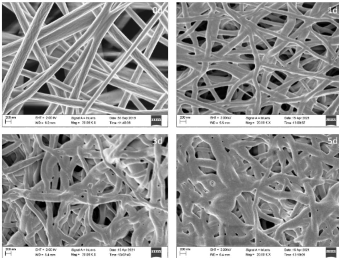
**Figure 2.** SEM of PαAPz-F fibers mat after degradation for day 0, day 1, day 3, and day 5.
